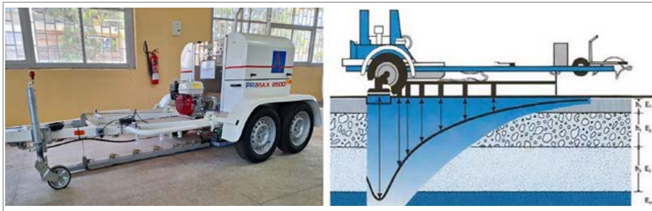
Figure 8.12 Illustration of FWD Equipment (TRL, ORN 18)
