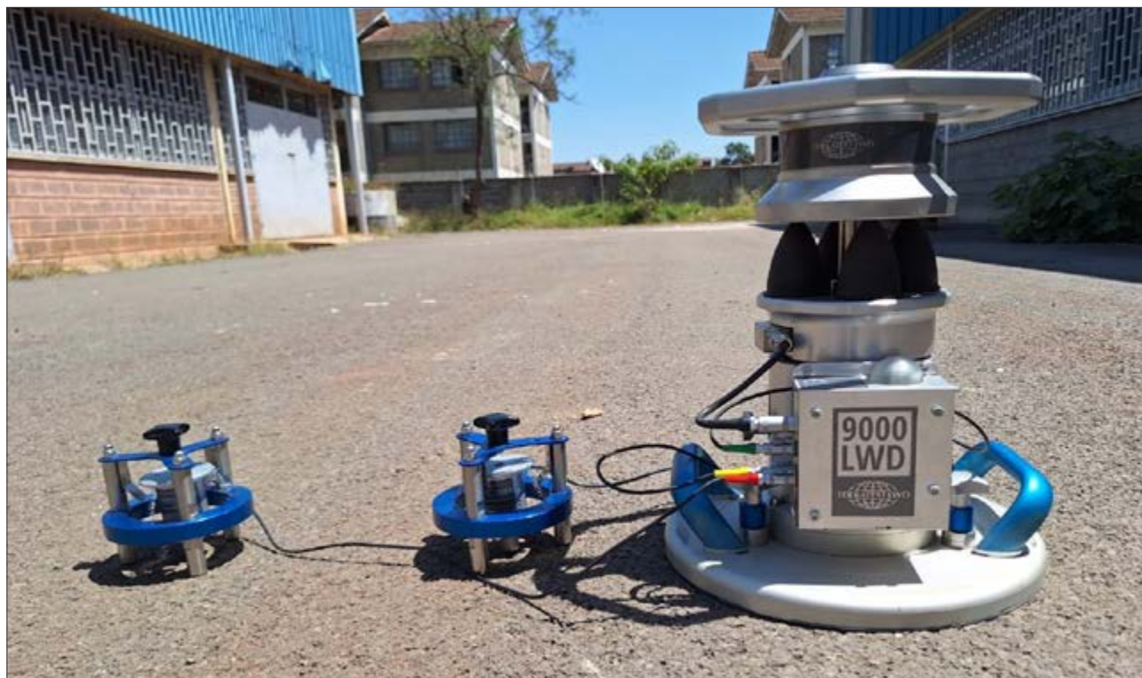
Figure 8.19 Light Weight Deflectometer (LWD) Complete with Additional Geophones
