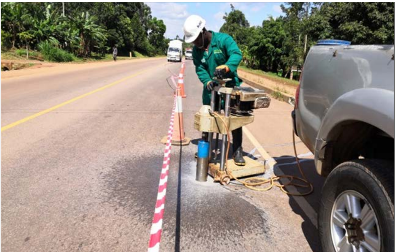
Figure 8.22 Coring of Asphalt Layers
