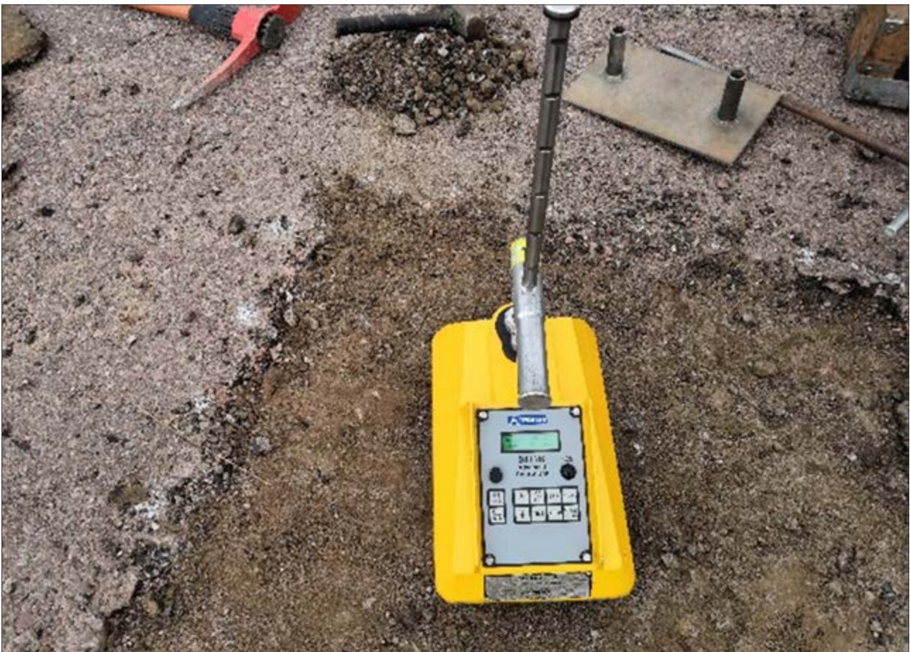
Figure 8.26 Measuring Field Density using a Nuclear Density Gauge
